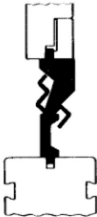
Typical power break forming tooling. Dies shown in blue.
